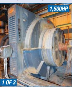
ELECTRIC MACHINERY Brushless Synchronous Motor
