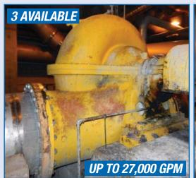
AHLSTROM Z-X70V-2 Split Case Fan Pump
