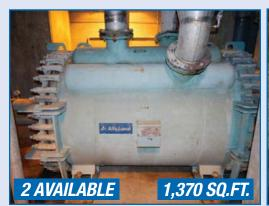
ALFA LAVAL Spiral Heat Exchanger
